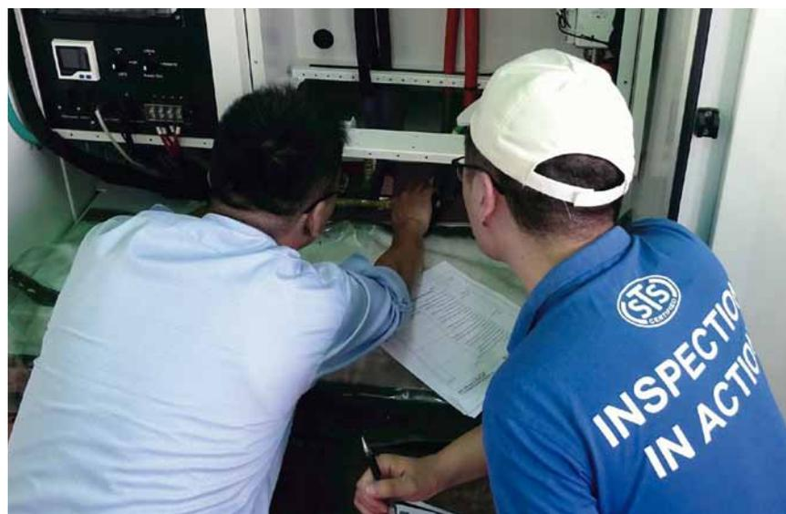
An inspector witnesses an STS functional test at an ESS factory.
